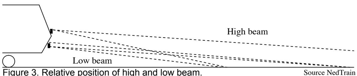
Figure 3. Relative position of high and low beam.
