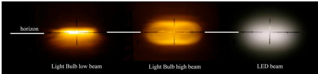
Figure 4. Luminous intensity of bulb and LED beams.
